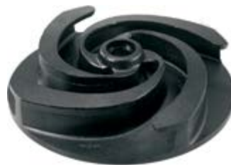
Vortex impeller. The vane winglets prevent the formation of secondary eddies over the vane edges, improving pump efficiency.
