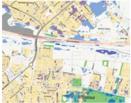
Backflow map showing the result of an extreme rainstorm incident. The blue areas are flooded with water after a high-intensity rainstorm event.
