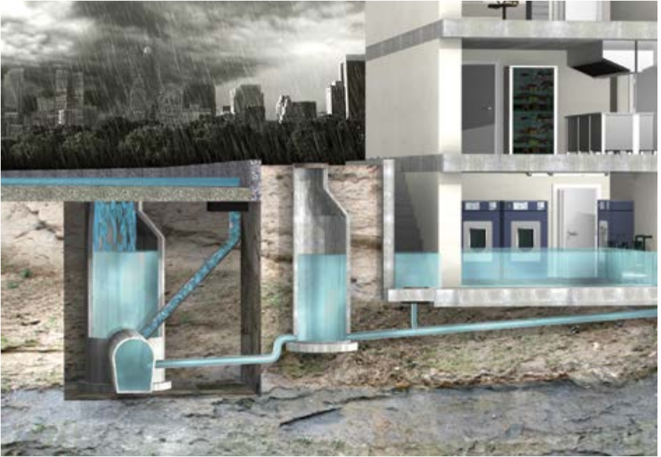
Water backflow event where an unprotected basement is flooded. In this situation, the building must be evacuated as the sanitary system is out of use.
